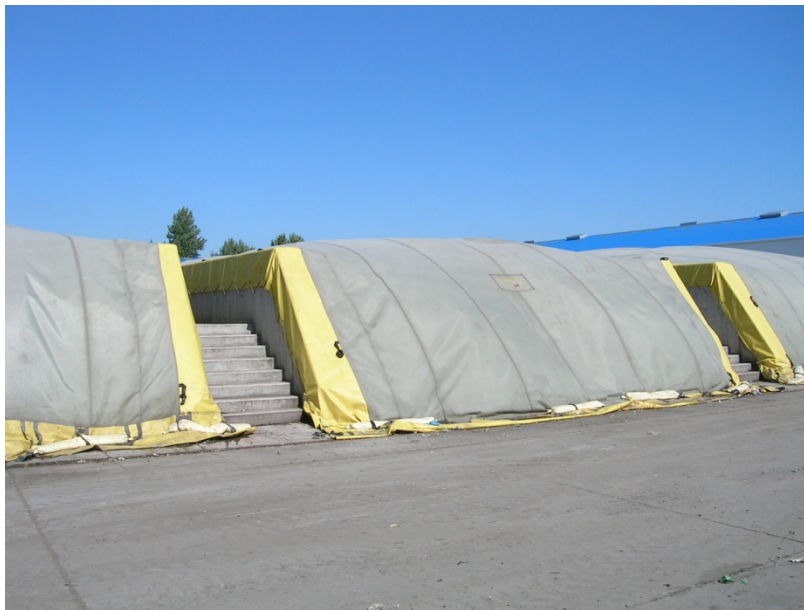
Figure 7. Covered MSW with semipermeable film
