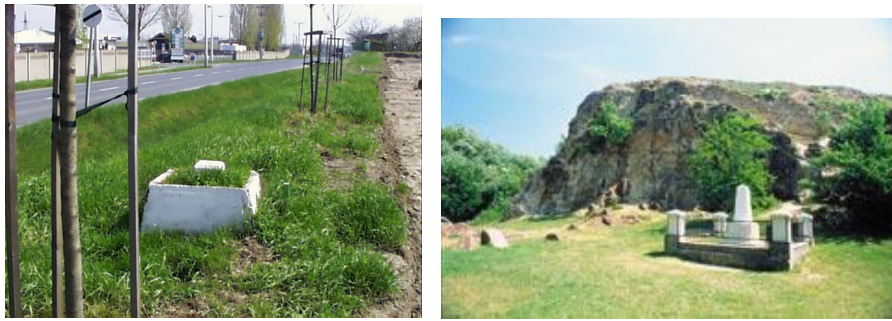
Figure 5.2. 4-order control point (left) and leveling point of reference, Nadap (right)
